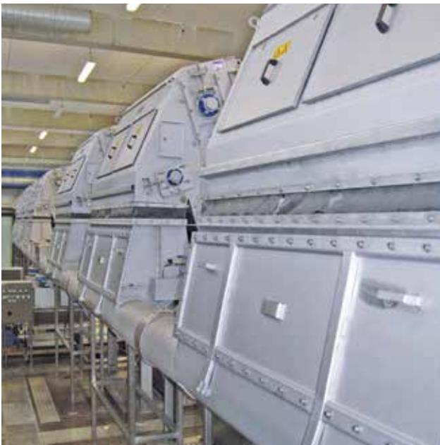
Rear view of the HUBER Belt Screen EscaMax® with subsequent launder channel for wear-free screenings transport.
