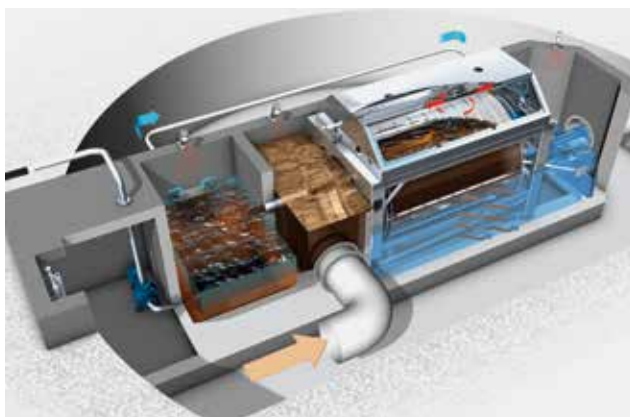
CarbonWin® process illustration: The better preliminary clarifier tank for optimum reduction rates (see individual brochure).
