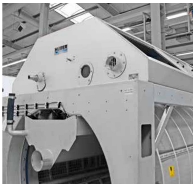
Polyurethane sealing in the inlet of the HUBER Drum Screen LIQUID.
