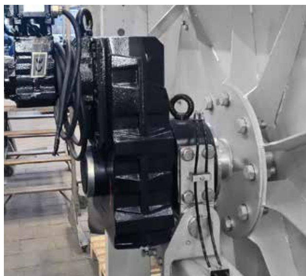
Low-maintenance chain drive on the HUBER Drum Screen LIQUID.
