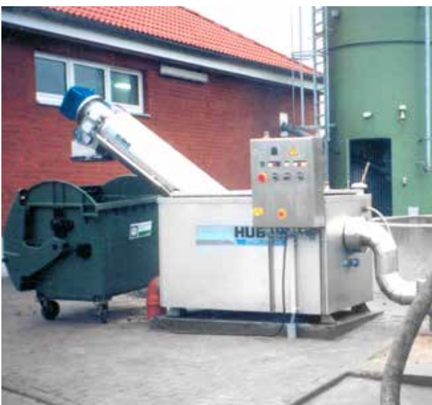
HUBER Sludge Acceptance Plant ROTAMAT® Ro3.1 with HUBER Fine Screen ROTAMAT® Ro1, heated and insulated unit.
