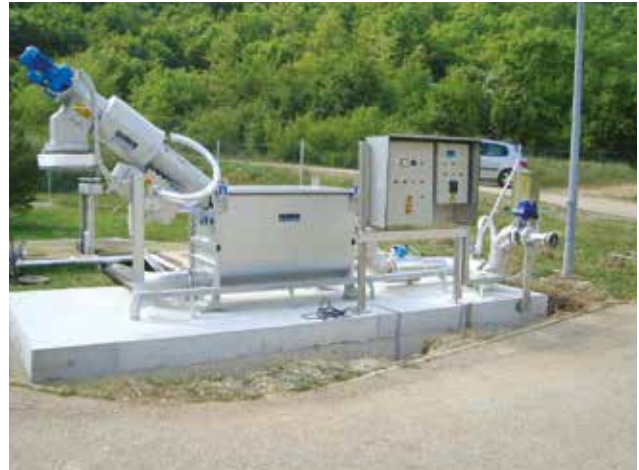
HUBER Sludge Acceptance Plant ROTAMAT® Ro3.1 with HUBER Fine Screen ROTAMAT® Ro1.
