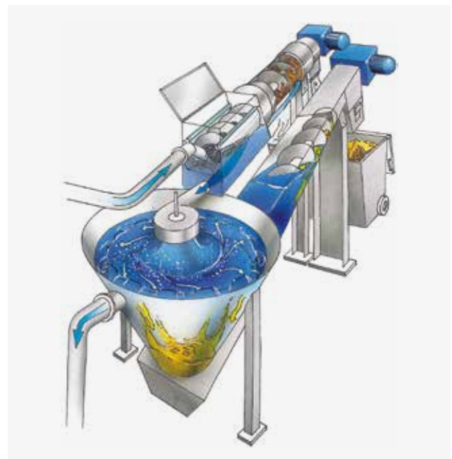
Schematic drawing of a HUBER COANDA Complete Plant ROTAMAT® Ro5 C.
