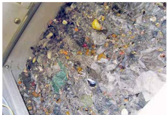
HUBER Fine Screen STEP SCREEN® SSF: The high separation efficiency is achieved through the narrow slot width and the produced screenings carpet. The self-cleaning effect is ensured by movable lamellae.
