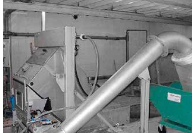
HUBER Fine Screen STEP SCREEN® SSF with HUBER Wash Press WAP® for optimal separation and dewatering results. Acid treated in a pickling bath for corrosion protection.
