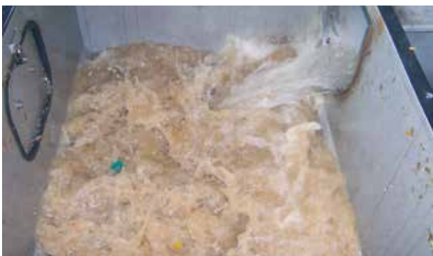
High turbulence in the launder tank during impeller operation.
