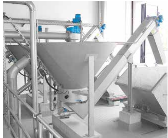
Reduced disposal costs and improved hygienic conditions with the HUBER Coanda Grit Washer RoSF4.
