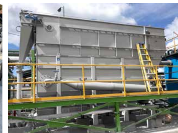
HUBER Dissolved Air Flotation for physical-chemical pre-treatment – optimum reduction of COD, fats and solids, more than 500 installations worldwide.
